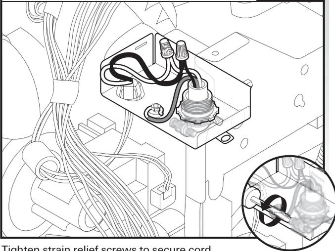
Tighten strain relief screws to secure cord.
